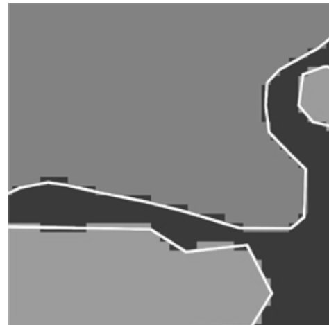
Fig. 4.7b: Magnified Views of the Same GIS Data File Converted into Vector Format.
